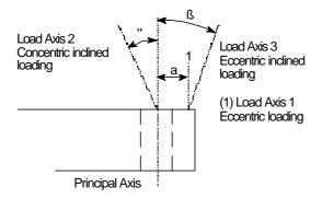
Fig.7 Eccentric and angular loading
