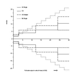
Fig.5 Combined error comparison
