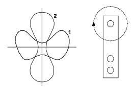
Fig.9 Specific eccentric loading diagram of an SHBxR (1) and SSB (2) type load cell, showing the error experienced at defined eccentric angular positions.
