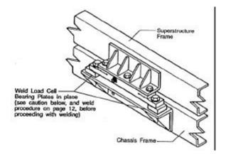
Fig. 12: Positioning before welding
