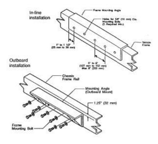
Fig. 9 Mounting the brackets
