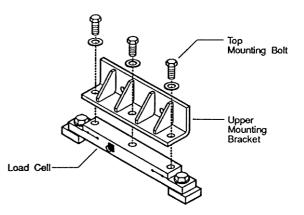
Fig. 10: Assembly of MWP and brackets
