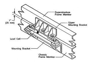
Fig. 5: Outboard mounted load cell
