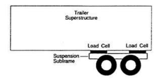
Fig. 3: MWP trailer installation
