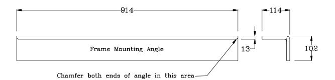
**NOTE:** At the installer's option, mounting angles for in-line installations may be fabricated the same as outboard mounting brackets shown on page 8, except without gussets.
