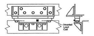
Fig. 6: Inverted installation
