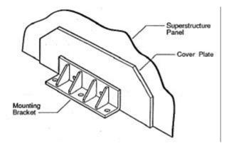
Fig. 8: Mounting bracket with a cover plate
