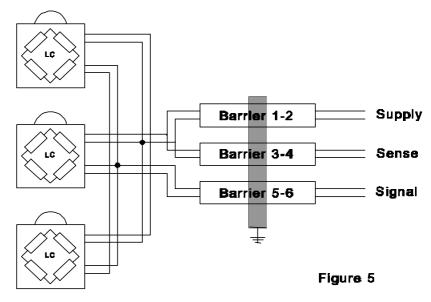
Figure 5: Basic system configuration with four-wire load cells. The cable forms part of the temperature compensation circuit of the load cell and should never be cut.
