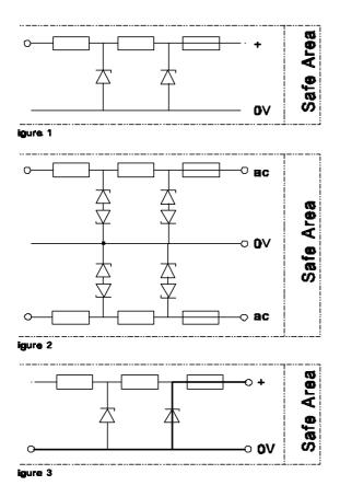
There are three basic types of simple resistive passive barriers used for standard weighing installations. A barrier which will sustain a positive voltage with respect to the 0 V is called a positive barrier and is configured as shown in figure 1.
