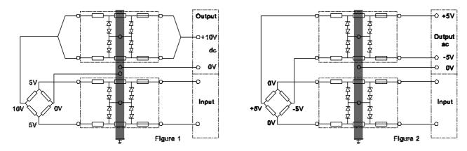
Figure 1 shows a non-balanced or basic bridge circuit. A voltage of 10 Vdc is applied to the bridge, which will result in a potential of 5 V on each output line in a no-load situation. The voltage between the two output lines will be 0 V. In the case of a 2 mV/V load cell at full load, the potential at one output line will decrease to 4.99 V and the potential at the second line will increase to 5.01 V. The voltage between the two output lines will then be 0.02 V = 20 mV.
