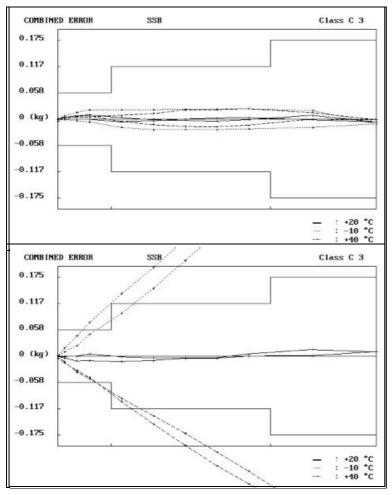
The graph opposite shows the result of a temperature test performed on a SSB type load cell with a maximum capacity of 500kg.
