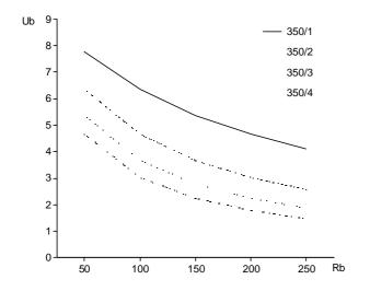
The diagram shows the operating voltage of the load cells, when a barrier channel with end-to-end resistance Rb is introduced in each line, at an excitation of 10 V, supplied by the indicator.
